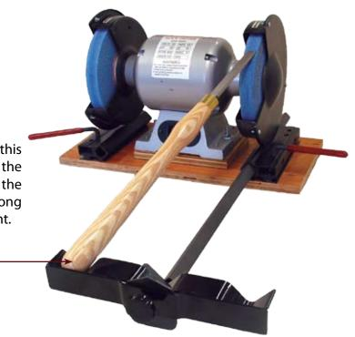
When the one side is done flip the tool over and put the handle in the right pocket with the short point to the right. Repeat the grinding procedure on this side.
